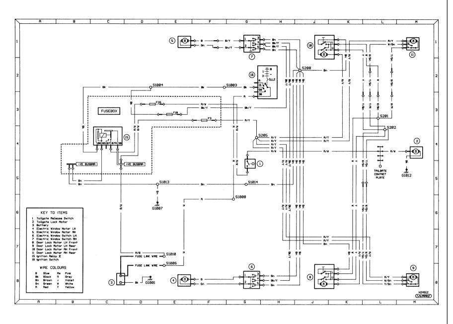
Diagram 3b: Ancillary circuits - central locking, electric windows and tailgate release (up to 1992)
